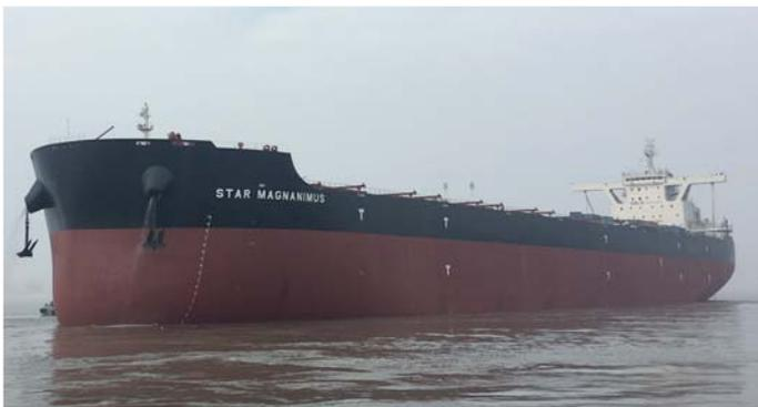
In March 2018, the bulk carrier *Star Magnanimus* was delivered to Greek shipowner Starbulk. This 208,000-DWT vessel is one of a series of 16 Newcastlemax ships that are currently being built to Bureau Veritas class in the Chinese shipyard Shanghai Waigaoqiao. With an overall length of 300 meters and a beam of 50 meters, *Star Magnanimus* will rank among the largest vessels capable of entering Newcastle port in Australia.
